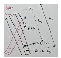
$$\overline{x} = \frac{M \times \frac{1}{2}L + mb_1 + mb_2}{M + 2m}$$
